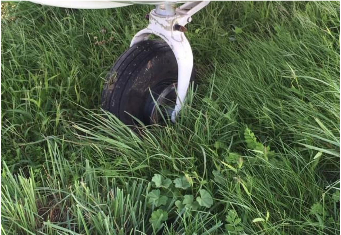
Fig. 6. The nose wheel punctured tyre and damaged wheel-hub at the aircraft's final resting position.
