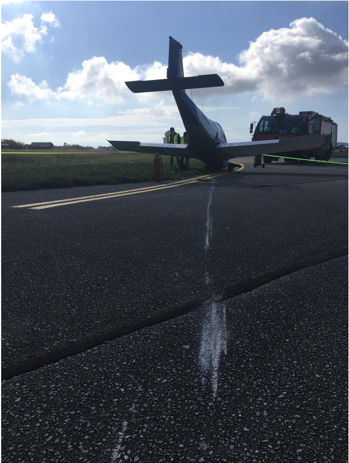
Fig. 5. Scratch marks on the ground close to the aircraft's final resting position.
