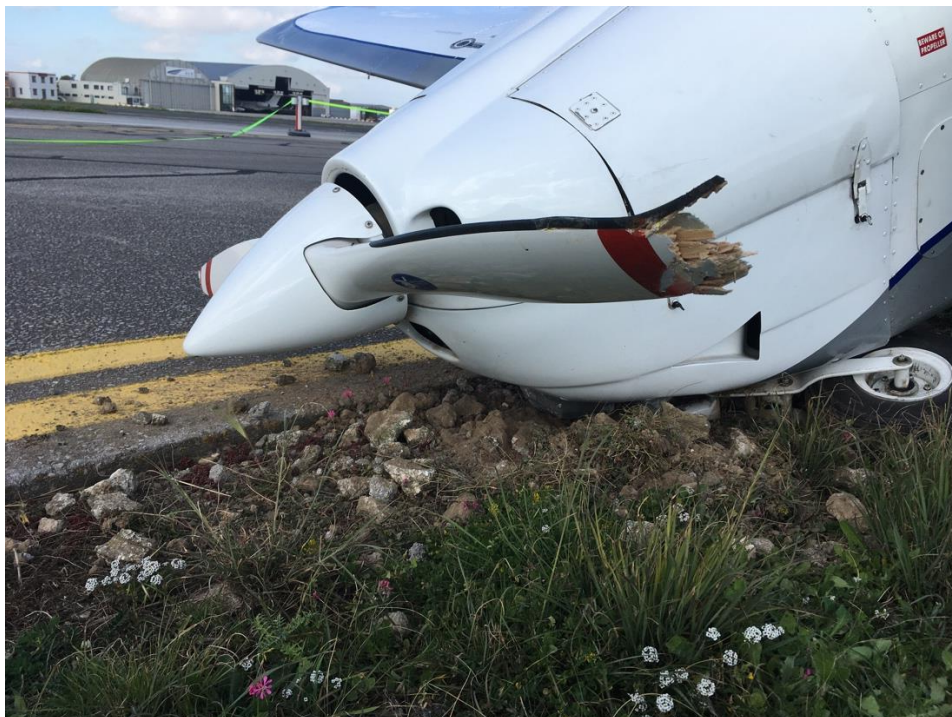
Fig. 6. Nose wheel collapse and damaged propeller.
