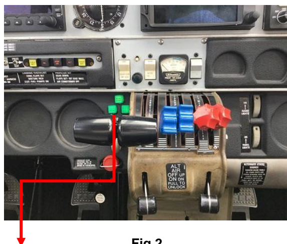
Fig.2 3 Greens on the Landing-Gear down and locked indication.
