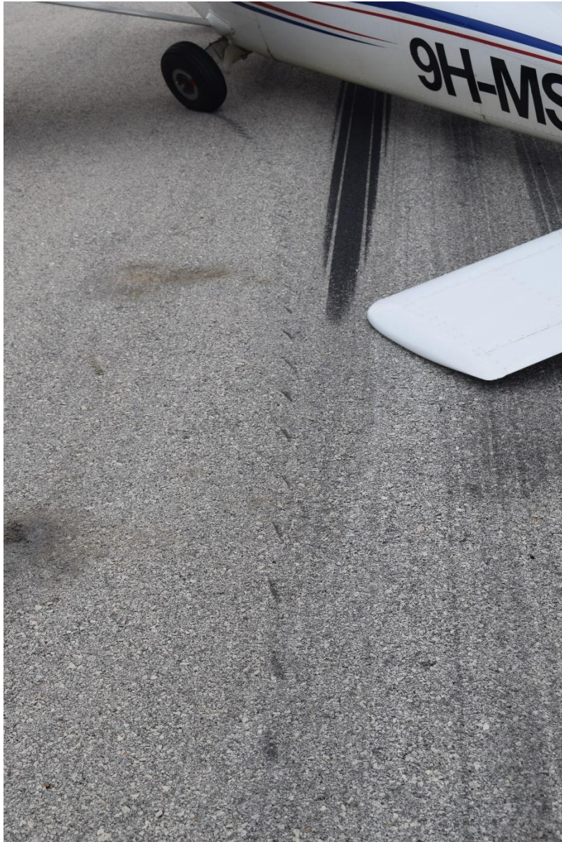
Figure 3. The left main undercarriage leg of the accident aircraft and the tyre marks generated by the left main undercarriage immediately prior to coming to a halt.
