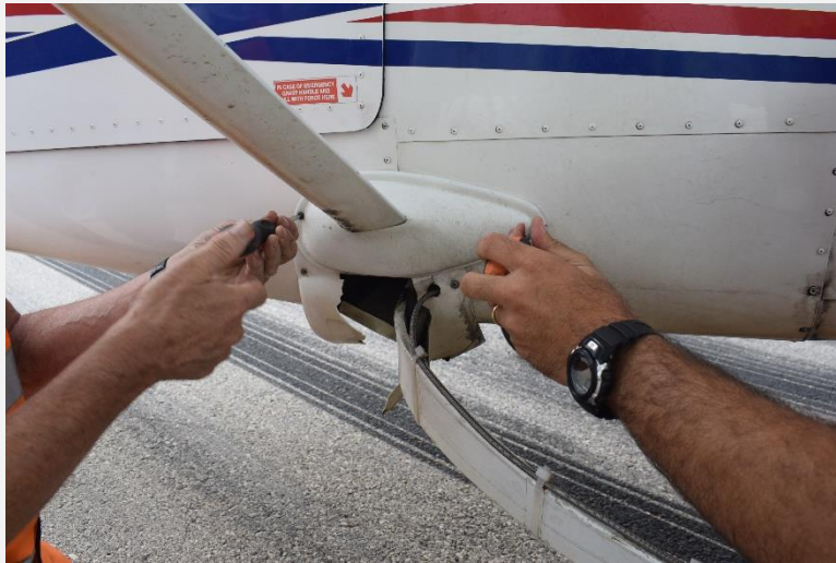
Figure 5. The collapsed left main undercarriage leg showing the leaf spring turned backwards.
