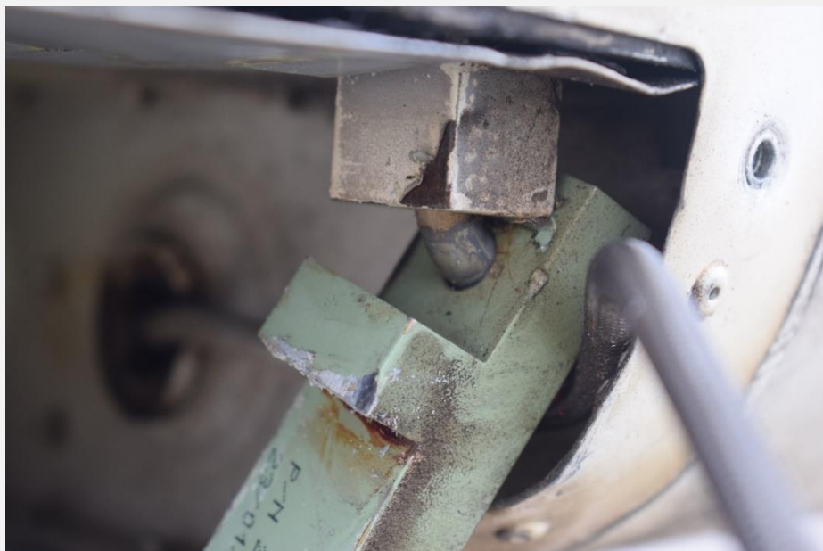
Figure 8. The rear outer bolt, as found following the accident, bent by the clamp on the collapse of the undercarriage leg.
