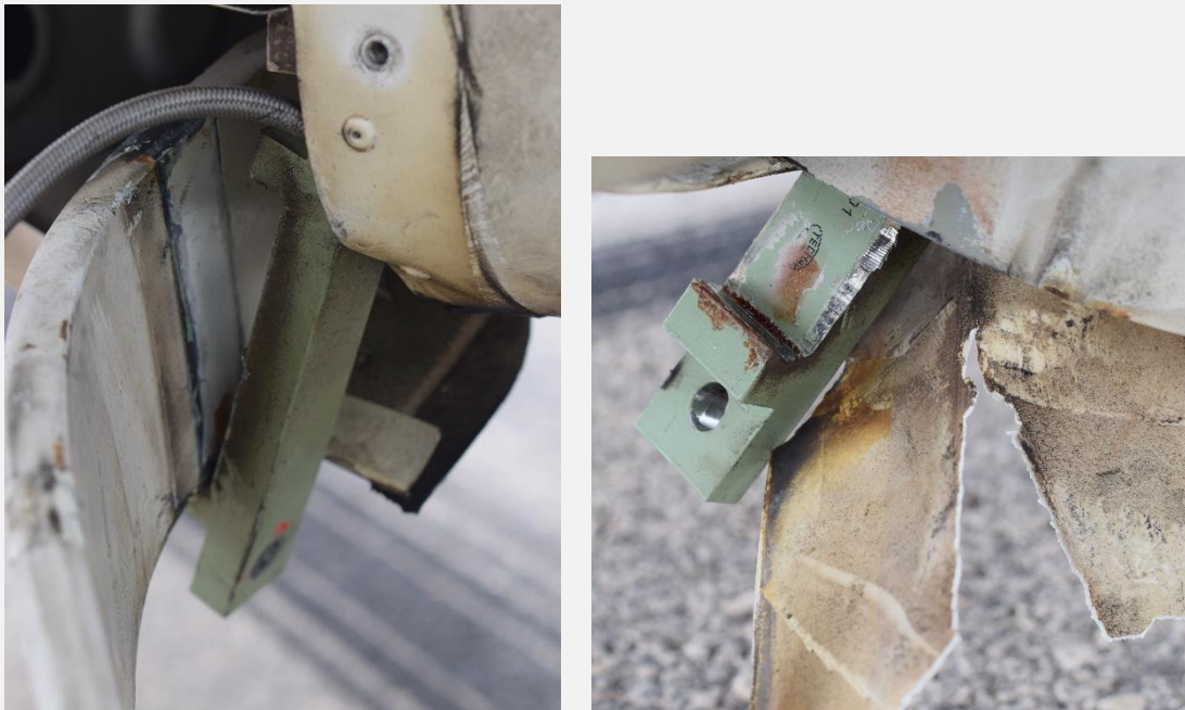
Figure 6. Views of the collapsed left main undercarriage leg following the accident, showing the clamp (green) pulled off the front outer bolt.
