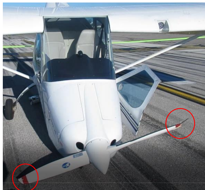
Fig. 2 Damage to the propellers and underside of the aircraft
