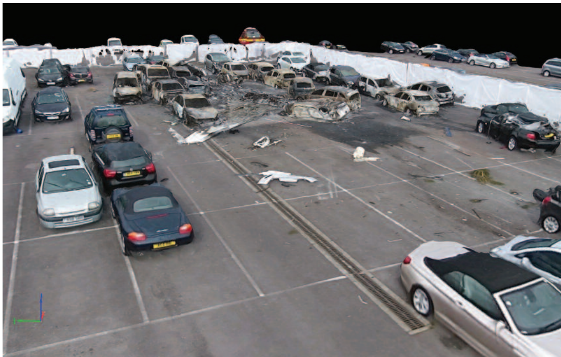
Figure 5: 3D mesh created from oblique video from Phantom 2 Vision Plus while flying two circles at two different heights around the main wreckage
