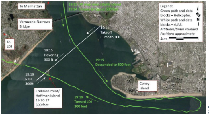
© NTSB Collision between Sikorsky UH-60 Black Hawk helicopter and DJI Phantom 4 drone
