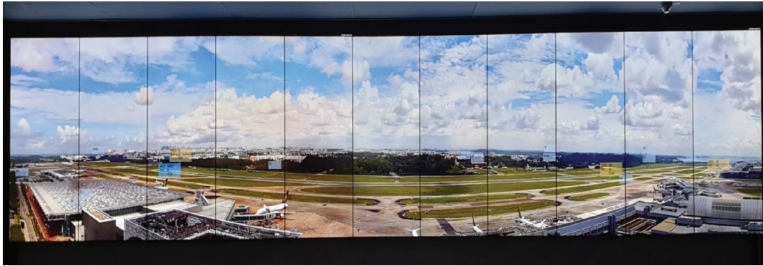
Smart Digital Tower – video wall with a runway view
