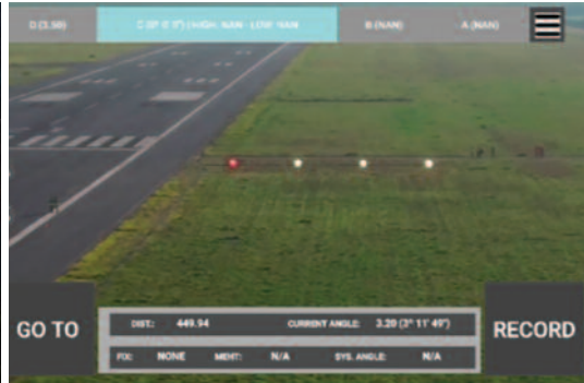
PAPI Calibration, RPAS + artificial intelligence.
