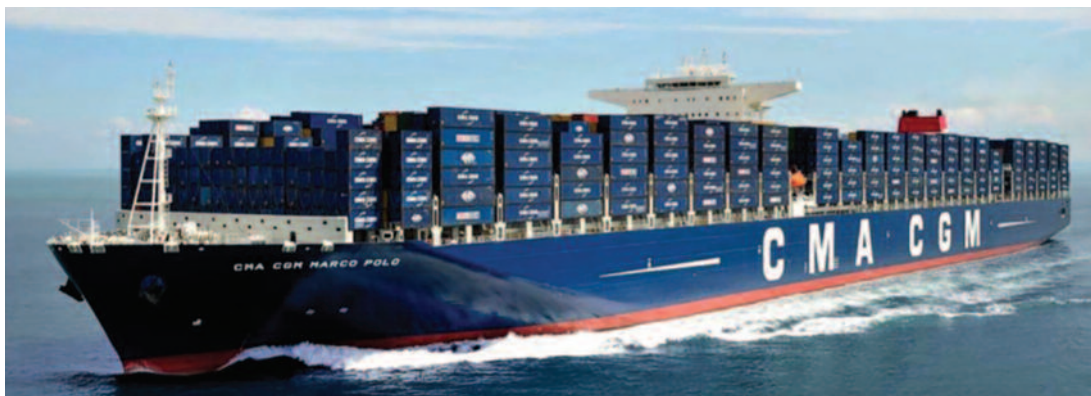
Larger container ships – increases energy efficiency through increased transport work for same or less energy consumed
