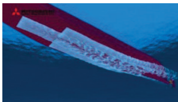
Illustration shows the air bubbles produced by the Mitsubishi Air Lubrication System (MALS) system. Illustration credit: MHI
