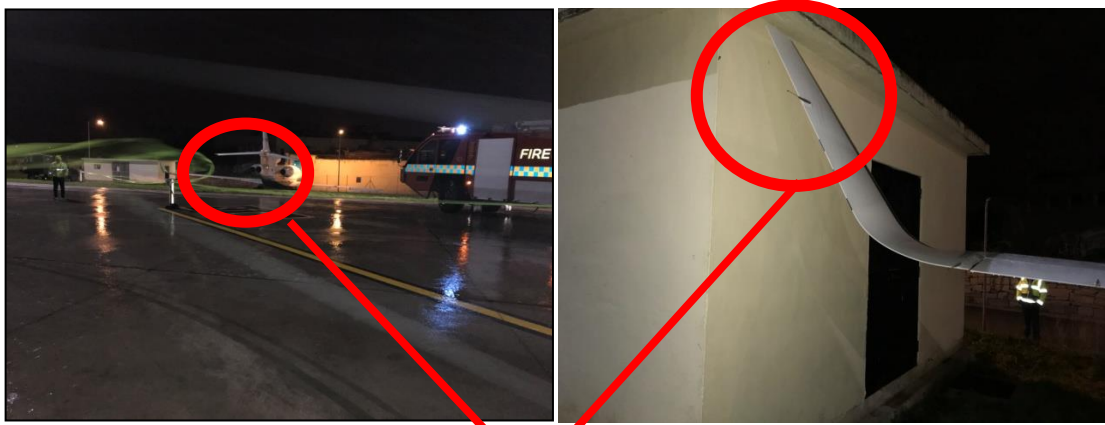
Fig.5. A photograph showing how the left winglet missed the High Voltage Distribution Centre wall by approximately 4 centimetres.
