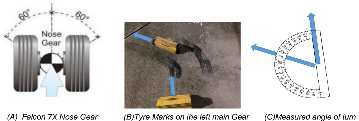
Fig. 4B. Photographs of the chocks as found on-site
