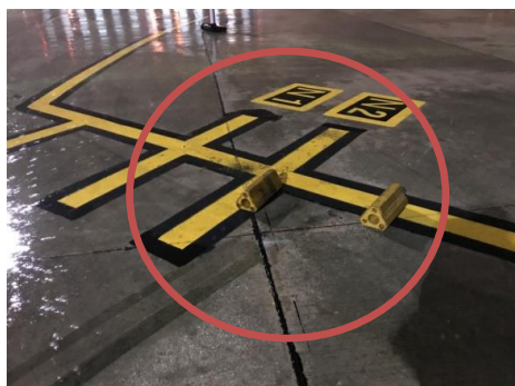
Fig. 7. Show the Nose-Wheel chocks as they were found after the accident.
