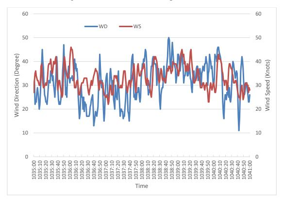
Figure 1.7-3 AWOS C wind speed/direction
