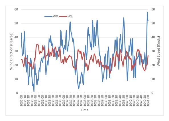
Figure 1.7-2 AWOS S wind speed/direction
