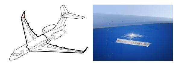
Figure 1.12-6 Middle bottom of the right winglet
