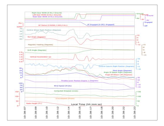
Figure 1.11-2 FDR readouts during landing phase (from RA 50ft)
