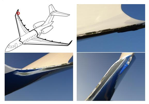
Figure 1.12-7 Trailing edge of the end of right wing An abrasion was detected on the right end of the aileron and split into two
