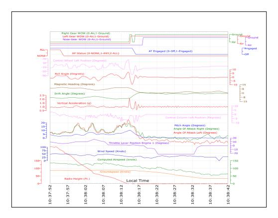
Figure 1.11-1 FDR readouts during landing phase (from AP disengaged)
