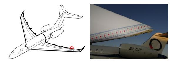
Figure 1.12-14 Left outboard flap fairing
