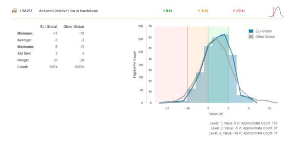
It is proposed that the LSA202 parameters be changed to reflect that airspeed on landing is approximately 5% less than Vapp / Vref. The proposed Event Parameters:
