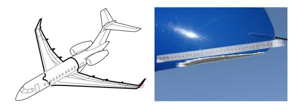
Figure 1.12-11 Trailing edge of the end of left wing
