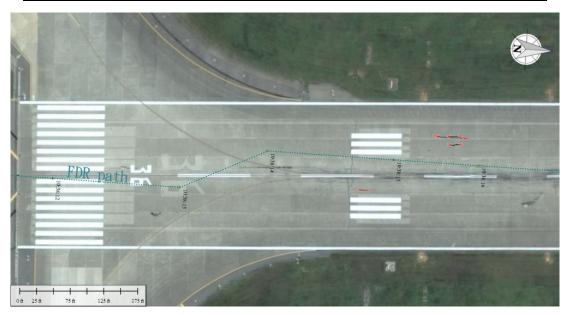
Figure 1.12-1 Superimposed site survey item and FDR flight path
