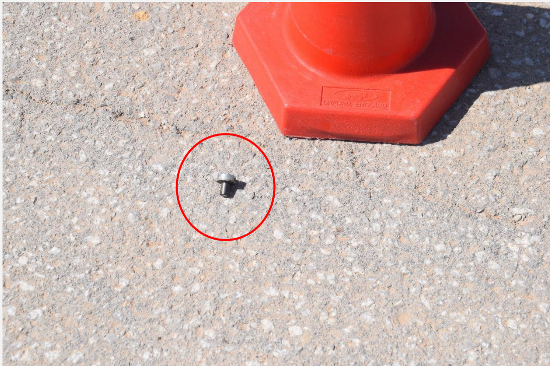
Figure 8: The head of the second shear pin found on TWY K (Kilo).
