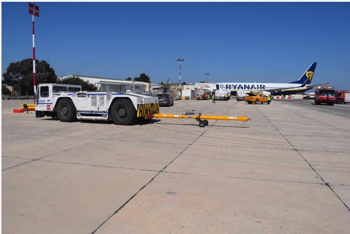
Figure 4: The Douglas DC10-4H tug and tow bar used in the accident event.
