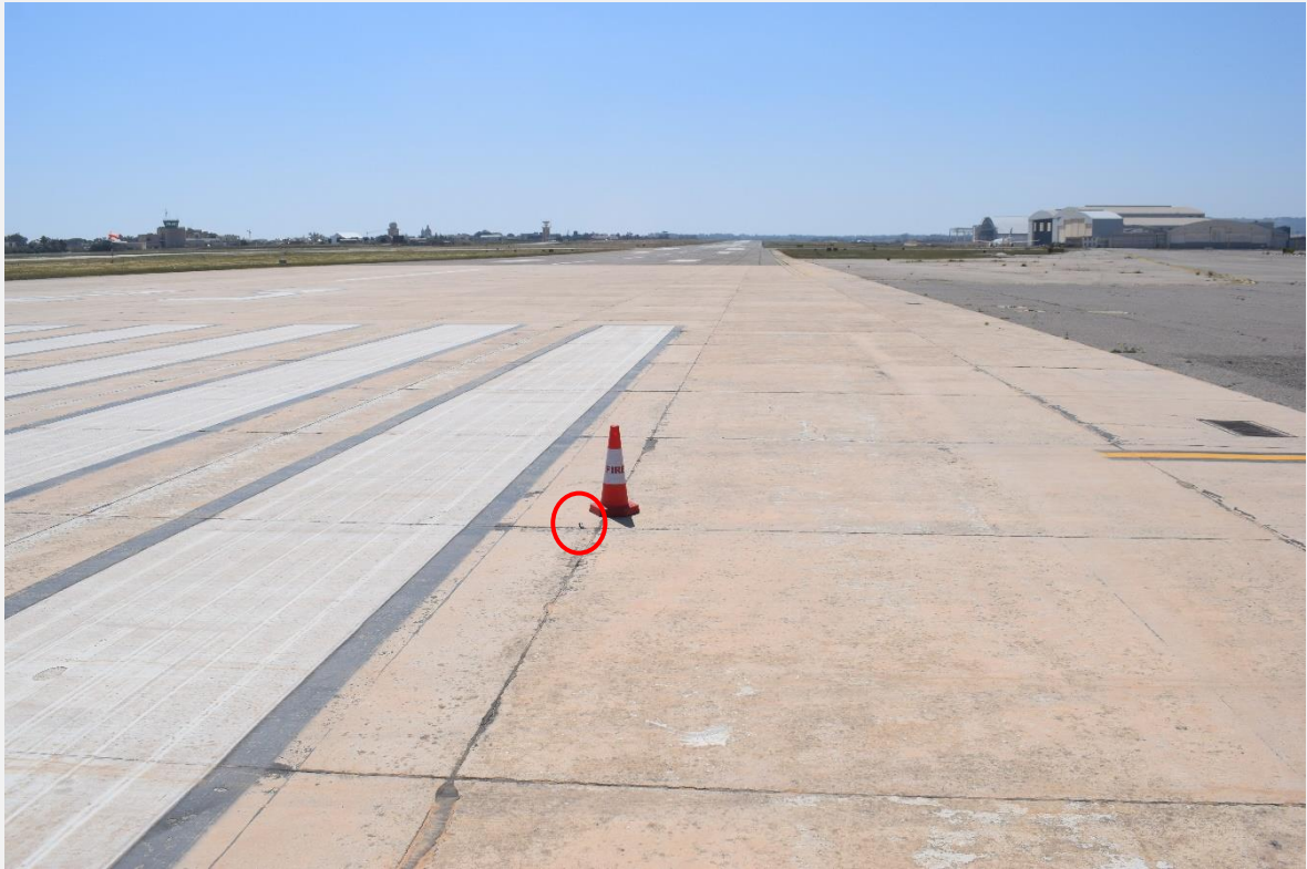
Figure 6: The remaining part of the retaining bolt (circled) found on RWY 23. The aircraft crossed the runway from left to right. TWY K (Kilo) commences just beyond the gutter.
