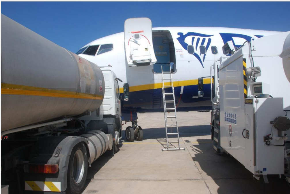
Figure 10: Exit Door L1 on the accident aircraft open.
