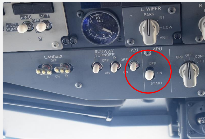
Figure 11: The APU switch found in the "ON" position during the field investigation.
