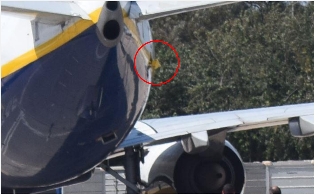
Figure 13: The APU inlet door in the open position with the APU shut down.
