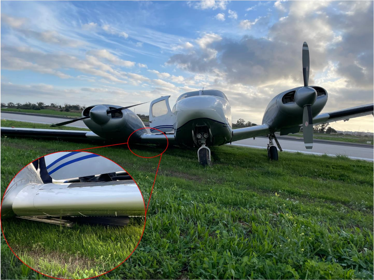
Fig. 2. The aircraft in its final resting position (nose view) with detail of un-extended landing gear
